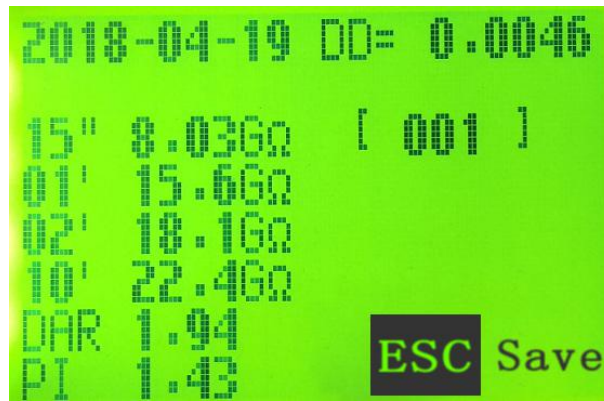
Measurement result storage (Figure 5)
