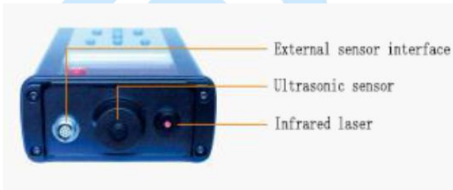
Fig. III Front End Layout of Host Machine
