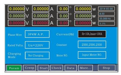
If the displayed parameter is the same with energy meter parameter, you do not need to set it anymore. Press the other function button to exit. Otherwise, click any color lump to set the energy meter parameter. See below picture:
