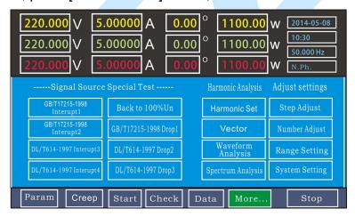
Press [vector diagram] button to enter vector diagram interface:
