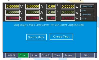
If it is mechanical meter, it needs catch black mark, press [marker]; set the test of grasping black mark.
