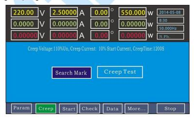
Voltage adjust to 220V, current adjust to 5\*50%=2.5A, when finish adjusting power source, each meter position shows [----], if grasp the black mark, it will shows [--1--]; when all meter position complete, press [--1--] to finish the work.
