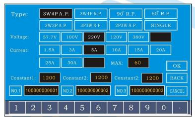
In the above picture, the first half part is parameter setting area, the middle is phase angle, and the last half area is number key
