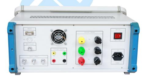
The five core aviation plug on the top left of back panel is the impulse output port of built-in standard meter, it can output standard meter's high frequency and low frequency. The middle RS232 is three line serial communications, can connect with computer; the three aviation plug on bottom left is the impulse input port of three tested energy meter. Other
