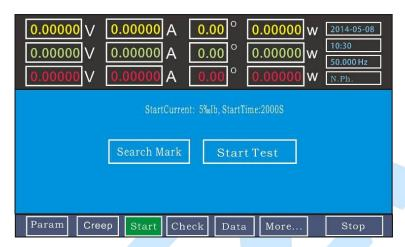
If to calibrate mechanical meter, it need to catch black mark, press [catch black mark] button;
