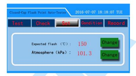
The interface can set expected flash point and the atmospheric pressure value: click "Expected flash" or "Atmosphere(kPa)" corresponding "change" into the expected flash point or pressure setting interface:
