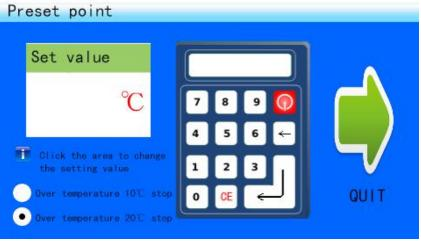
The interface, click "set value" region, keyboard expected flash point set value input box will show cursor, digital input and and confirm input by touch enter. To delete a
