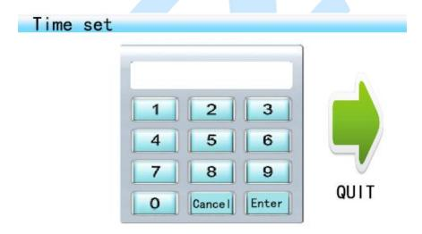
To adjust the date, time, click interface above the time display area, the keyboard input to revise time display (year, month, days, hour, minute, seconds position to use "?" to substitute, just follow the sequence. After input click Enter button to complete the change. If you quit, please click Cancel ".
