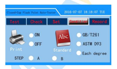
The interface is used to set the printer's opening, closing and testing standard, when set to "every degree", after the start of the test sample when temperature rise about  $5 \,^{\circ}\text{C}$ , the cover will open and ignite every time temperature increase  $1 \,^{\circ}\text{C}$  to test whether there is flash fire, it is applicable when the flash point of the specimen is not known.
