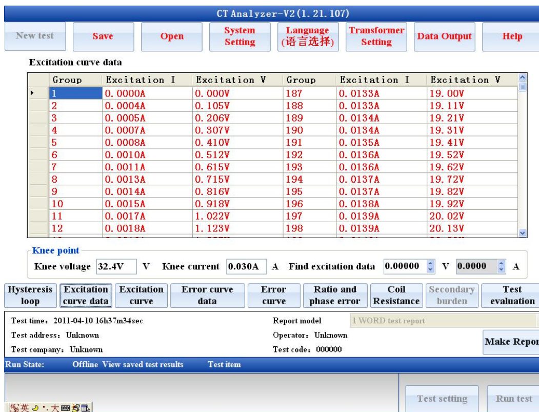
Figure 5.2 Excitation curve data
