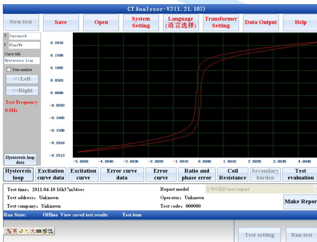
Figure 5.2.1 Hysteresis loop curve
