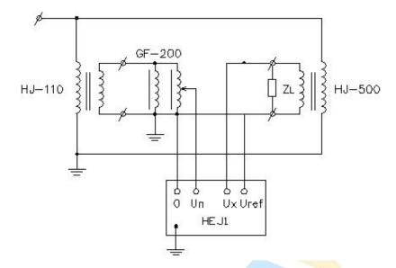
When the rated turns ratio of the the standard voltage transformer is not same with the test voltage transformer, here can use the induction divider to cascaded with the standard voltage transformer to measure the error of the detected voltage transformer.
