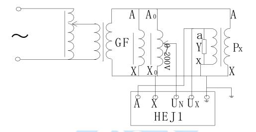
When the induction voltage transformer is used to check the voltage transformer, wiring connection is above. Here the accuracy standard error can be ignored, and the indication of the detected voltage transformer can be read out directly from the voltage transformer calibrator.
